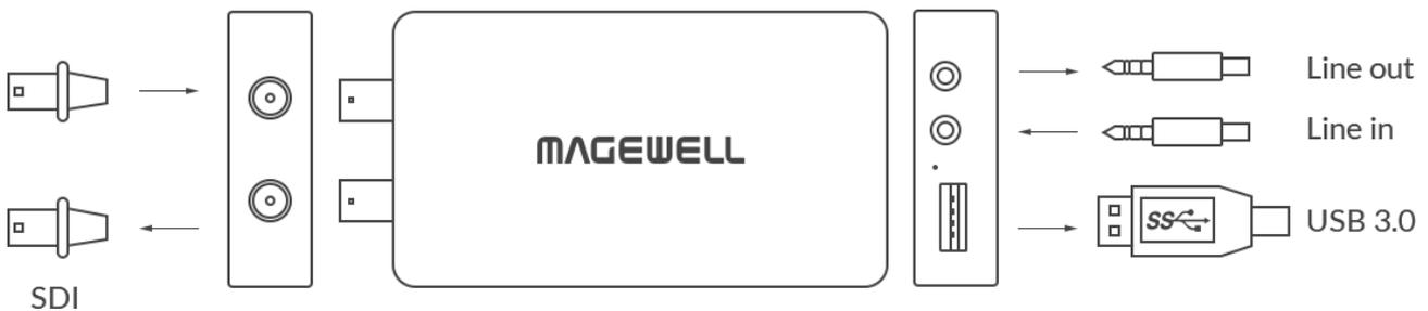
**MAGEWELL SDI Plus to USB Capture**, SD/HV/3G/ 2K SDI + embedded audio, Loop-through SD/HV/3G/2K SDI, Audio input via Line in, Extract SDI embedded audio and output via Line out
